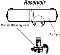
Figure 5-1 Manual Drain Valve
