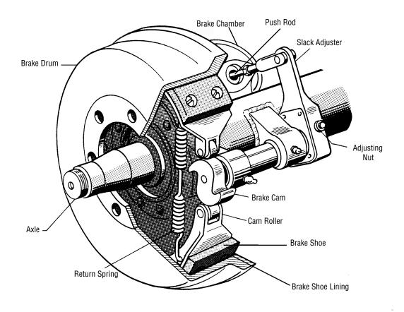
Figure 5-2 S-cam Air Brake
