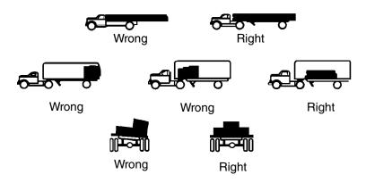
Figure 3-1 Balancing Cargo Weight
