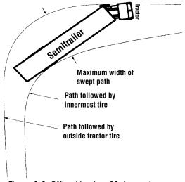
Figure 6-3 Offtracking in a 90 degree turn
