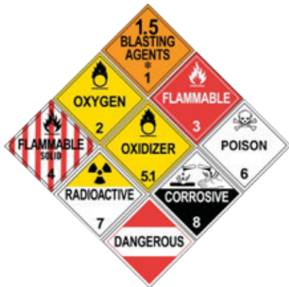
Examples of HAZMAT Placards Figure 9.3
