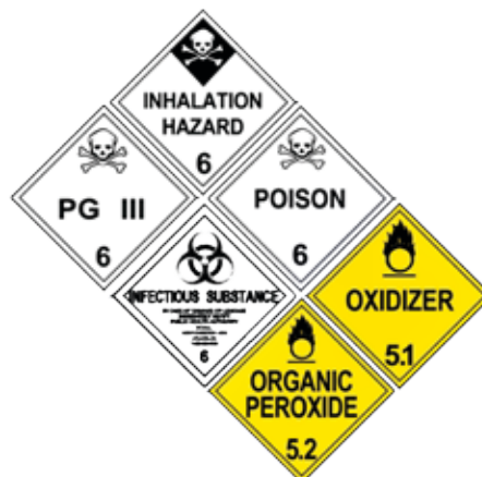
Examples of HAZMAT Labels Figure 9.2
