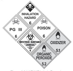
Figure 9.2 HAZMAT Labels Examples
