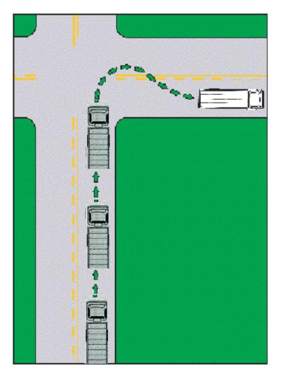
This illustration shows the correct procedure for making a right turn with a singleunit vehicle.
