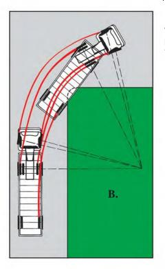
In illustration B, notice the rear wheels of the trailer follow shorter paths than the front wheels of the tractor.
