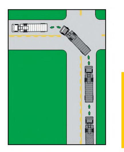
This illustration is the correct procedure for making a left turn with a tractor semitrailer. The procedure is the same with a single-unit vehicle.
