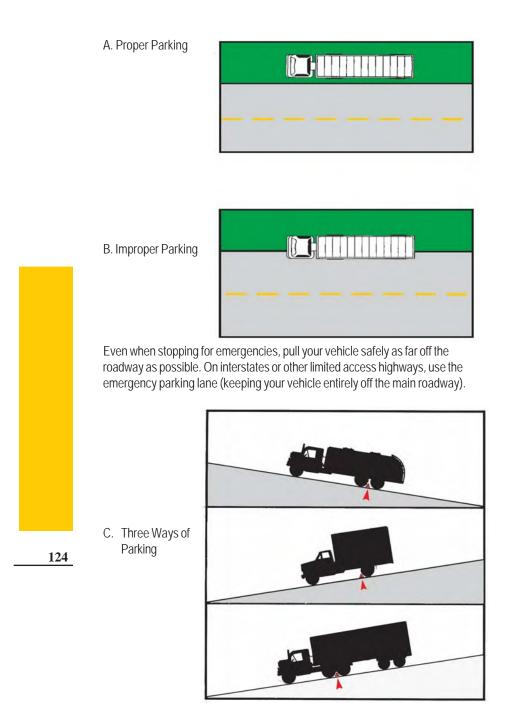
When parking on a hill, use chock blocks to reduce the chances of a runaway vehicle. Recommended placement of blocks indicated in red.
