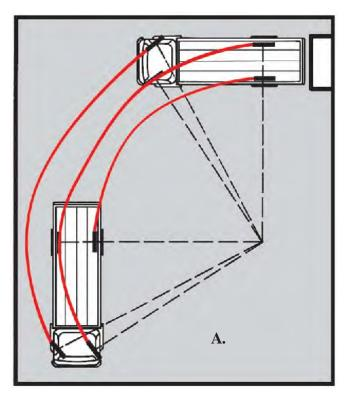
A. Steering (backing) with a single-unit vehicle
