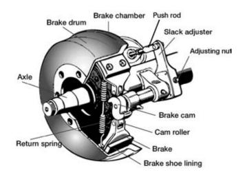
Brake drums are located on each end of the vehicle's axles. The wheels are bolted to the drums. The braking mechanism is inside the drum. To stop, the brake shoes and linings are pushed against the inside of the drum. This causes friction which slows the vehicle and creates heat. The amount of heat that a drum can take without damage depends on how hard and how long the brakes are used. Too much heat can make the brakes stop working.
