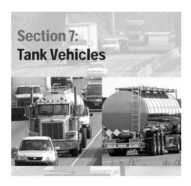
**A tank vehicle** is a vehicle used to carry any liquid or liquid gas in a tank of 1,000 gallons or more. A portable tank is a bulk container that is not permanently attached to the vehicle.
