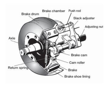
Brake drums are located on each end of the vehicle's axles. The wheels are bolted to the drums. The braking mechanism is inside the drum. To stop, the brake shoes and linings are pushed against the inside of the drum. This causes friction which slows the vehicle and creates heat. The amount of heat that a drum can take without damage depends on how hard and how long the brakes are used. Too much heat can make the brakes stop working.
