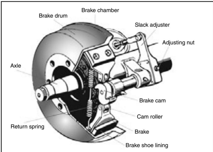
Figure 5.2, Drum brake
