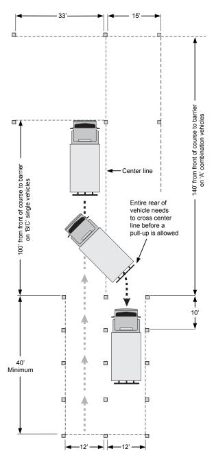
Figure 12.2 Offset backing to the right
