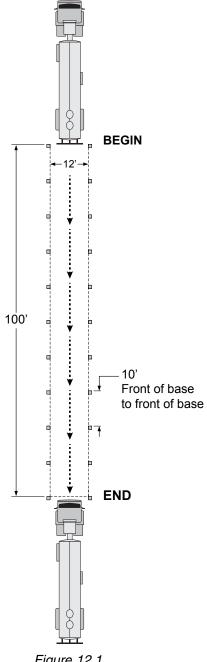
Figure 12.1 Straight line backing
