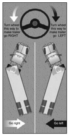
Figure 6.5 Backing a trailer
