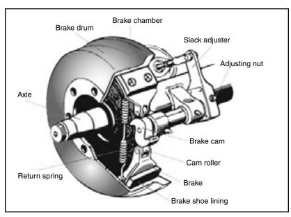
Figure 5.2, Drum brake
